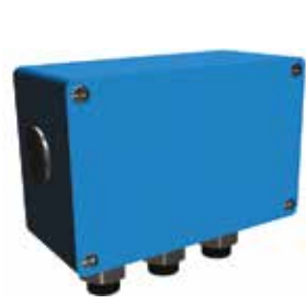
Small auxiliary aluminum terminal box for motor sizes 280-450 (variant codes 418, 568, 380, 569) The size of terminal box ordered with these codes depends on the number of accessories ordered. 80 x 125 mm, max 12 strips. Earthing size M4
