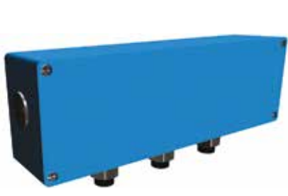
Large auxiliary aluminum terminal box for motor sizes 280-450. The size of terminal box ordered with these codes depends on the number of accessories ordered. 80 x 250 mm, max 30 strips. Earthing size M4
